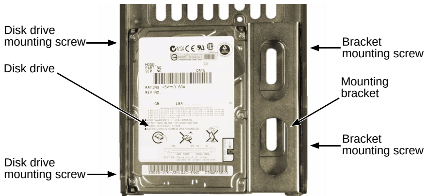
Figure 10. Drive carrier mounting screw locations
