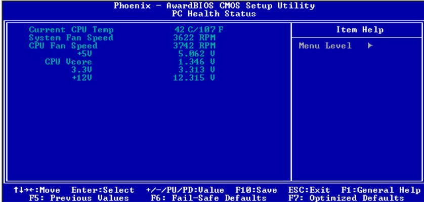
The PC Health Status displays the current status of all of the monitored hardware devices/components such as CPU voltages, temperatures and fan speeds.
