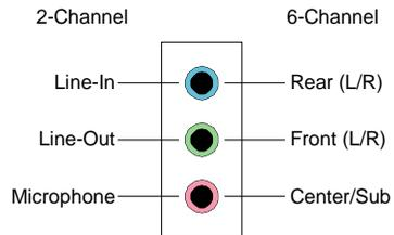
The **Mic** jack is for connecting to a microphone.
