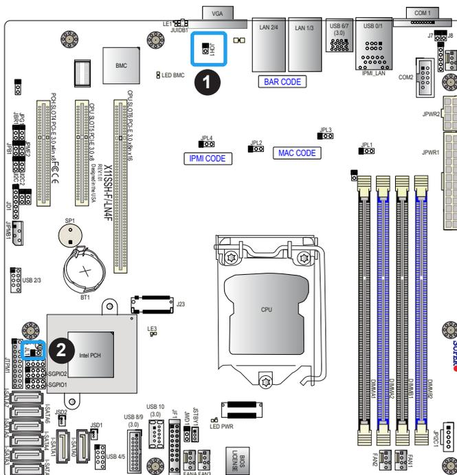
1. Overheat/Fan Fail LED Header
