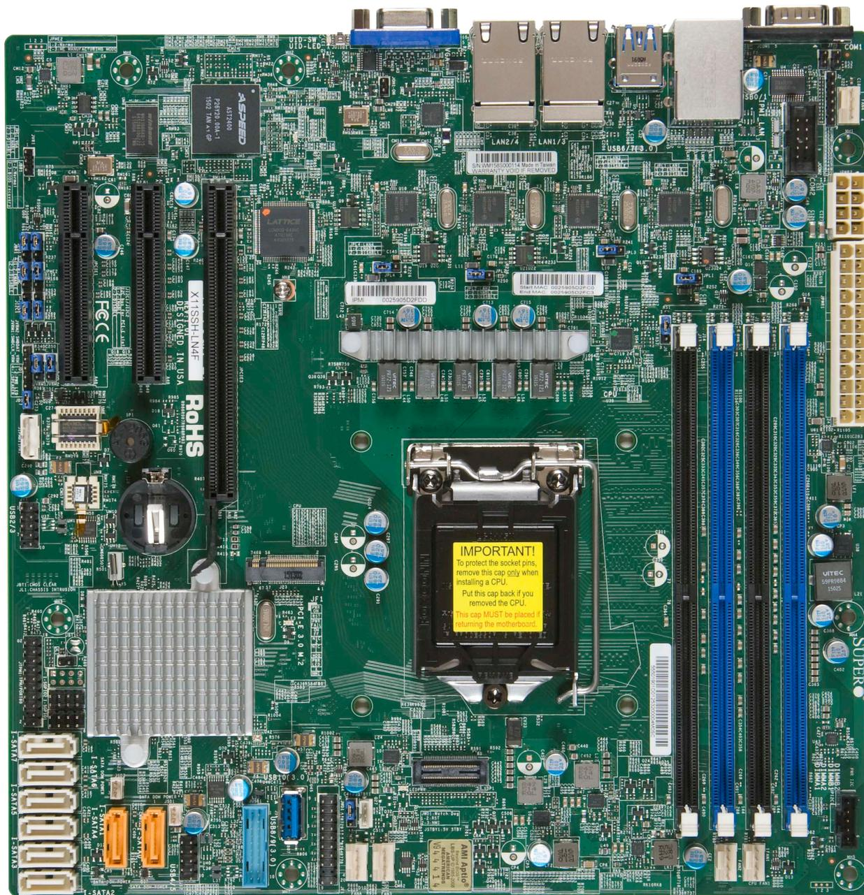
**Figure 1-3. X11SSH-F/LN4F Motherboard Layout**
