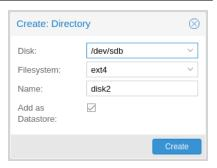
You can create an ext4 or xfs filesystem on a disk using fs create, or by navigating to **Administration** -> **Disks** -> **Directory** in the web interface and creating one from there. The following command creates an ext4 filesystem and passes the --add-datastore parameter, in order to automatically create a datastore on the disk (in this case sdd). This will create a datastore at the location /mnt/datastore/store1:
