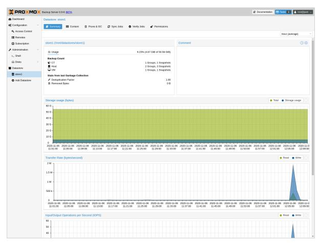
The Datastore section contains interfaces for creating and managing datastores. It contains a button to create a new datastore on the server, as well as a subsection for each datastore on the system, in which you can use the top panel to view:
