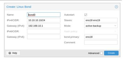
To add a new network interface, use the create subcommand with the relevant parameters. For example, you may want to set up a bond, for the purpose of network redundancy. The following command shows a template for creating the bond shown in the list above:
