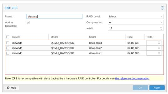
You can also create a zpool with various raid levels from **Administration -> Disks -> Zpool** in the web interface, or by using zpool create. The command below creates a mirrored zpool using two disks (sdb & sdc) and mounts it under /mnt/datastore/zpool1:
