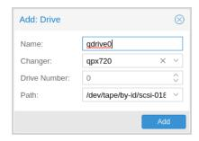
In order to use that drive with Proxmox, you need to create a configuration entry. This can be done through **Tape Backup -> Drives** in the GUI or by using the command below:
