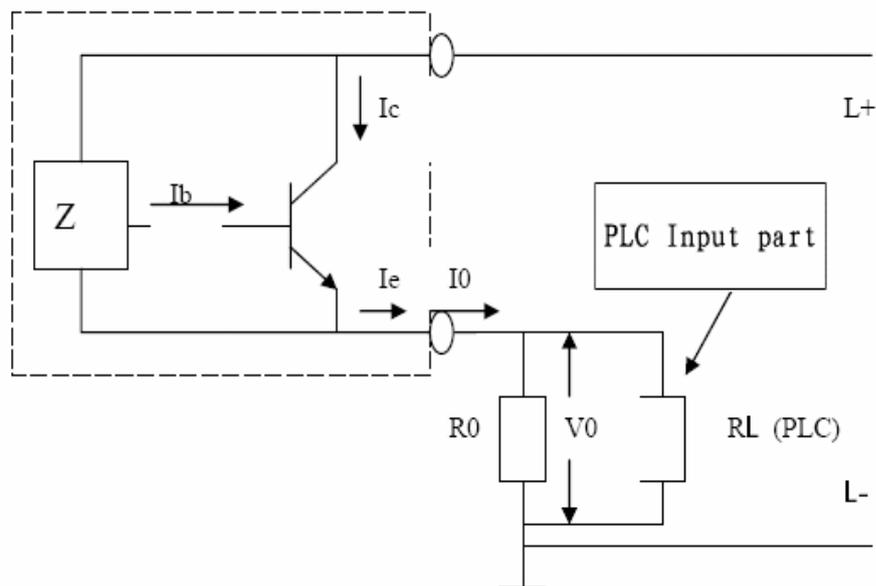
Analyze resistance  $R_0$  value and connection sensor with PLC:
