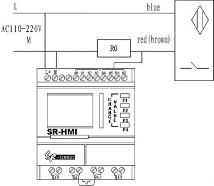
To the same type approach switch, its connection principle is alike. For NO and NC type approach switch, their difference is output relation when it near to the approach switch. For 3-Line AC, 4-Line AC and 2-Line AC, their difference is their connection methods.
