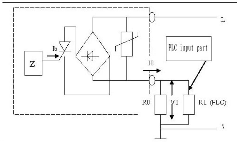
Analyze resistance  $R_0$  value and connection sensor with PLC
