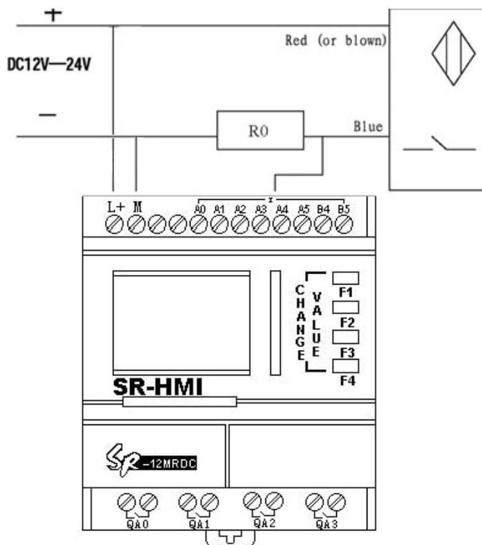
To the same type approach switch, its connection principle is alike. For NO and NC type approach switch, their difference is output relation when it near to
